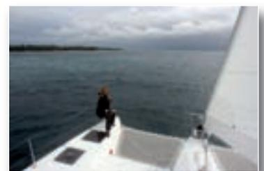
The false central hull reduces the area of the two trampolines. A configuration which is heavy, but helps with the platform's rigidity and the stowage capacity.
